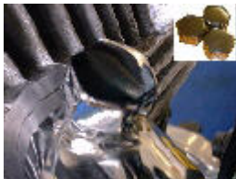
RI006 Emission blank nut - for hose connector on down-pipe when re- moving the PAV sys- tem. £4.50
